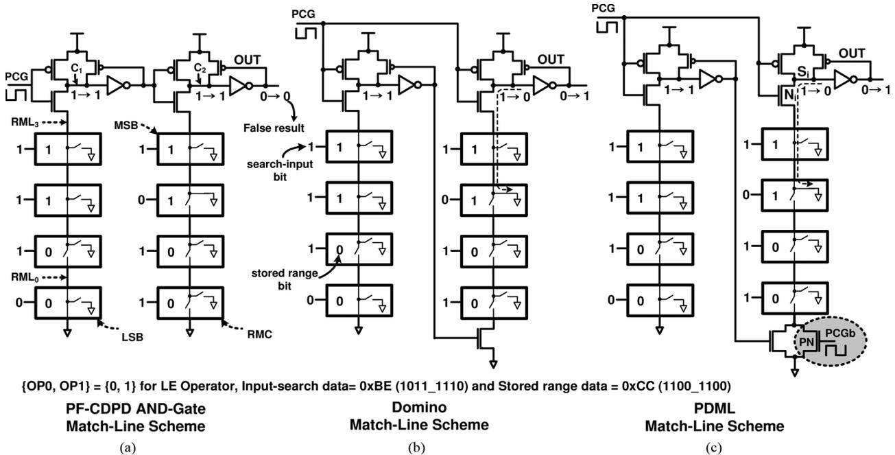
Fig. 7. Examples of range-matching in: (a) PF-CDPD, (b) domino, and (c) PDML match-line structures.
