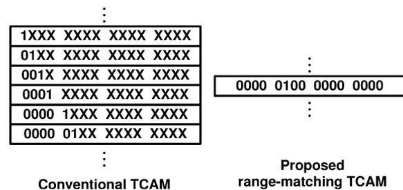
Fig. 1. Range mapping of the range 1024-65535 on a conventional TCAM and on a range-matching TCAM.
