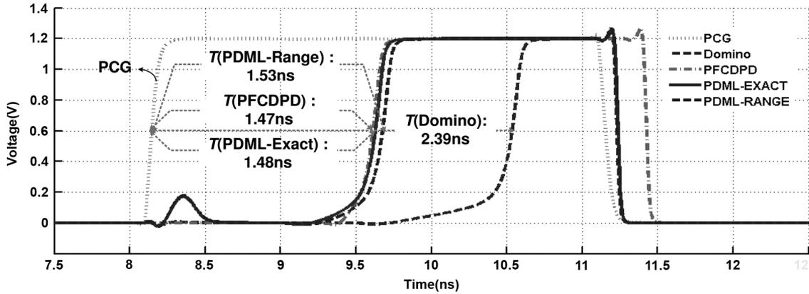
Fig. 10. Post-layout simulated waveform for full exact matching and RM in the worst case.
