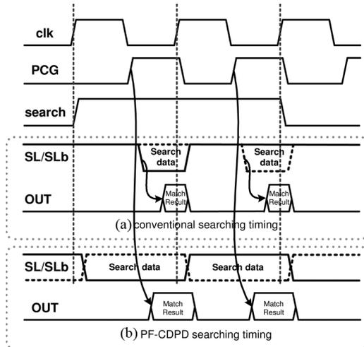
Fig. 8. Timing diagram of the search line. (a) Conventional method with search-line transition for precharging. (b) PF-CDPD method without search-line transition.
