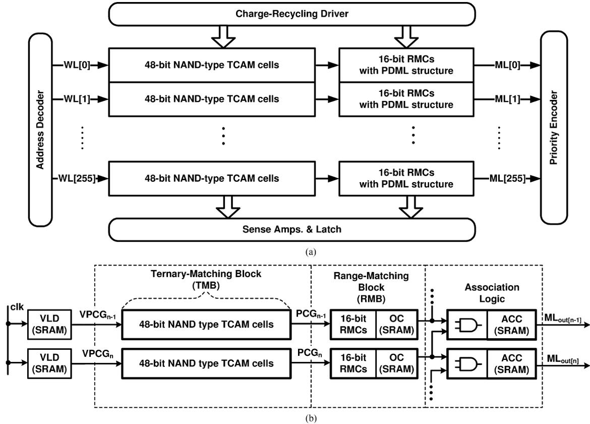
Fig. 2. (a) Block diagram of the range-matching TCAM. (b) 64-bit match-line structure of each entry.
