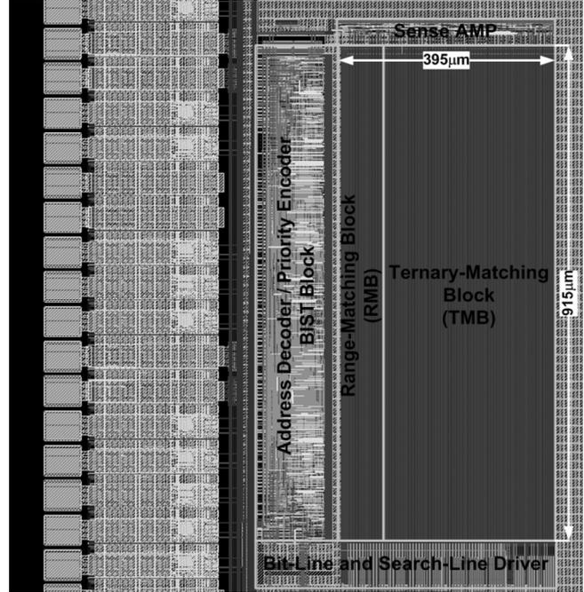
Fig. 12. A 256×64-bit layout of the proposed range-matching TCAM with dynamic match-line RMC and charge recycling-driver.
