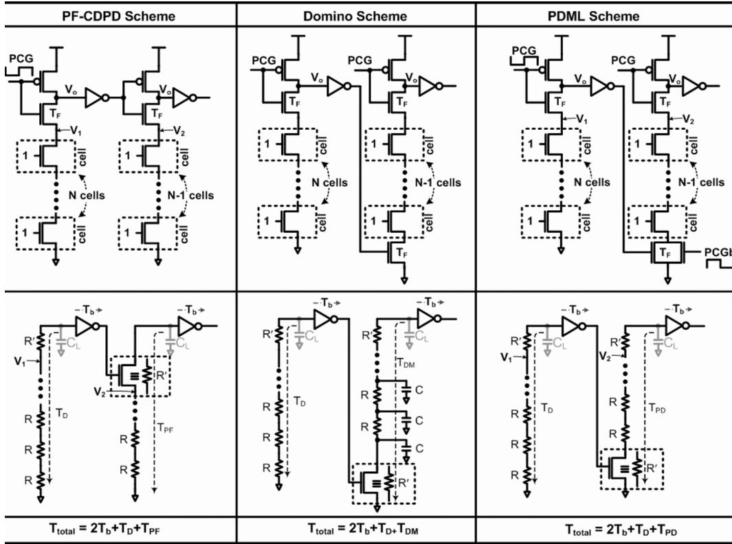
Fig. 9. Match-case evaluation and calculated delays of the PF-CDPD, the Domino, and the PDML schemes.
