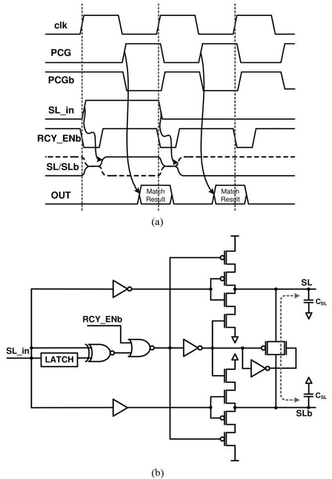
Fig. 11. (a) Timing diagram of the charge-recycling driver and (b) Circuit diagram of the charge-recycling driver.
