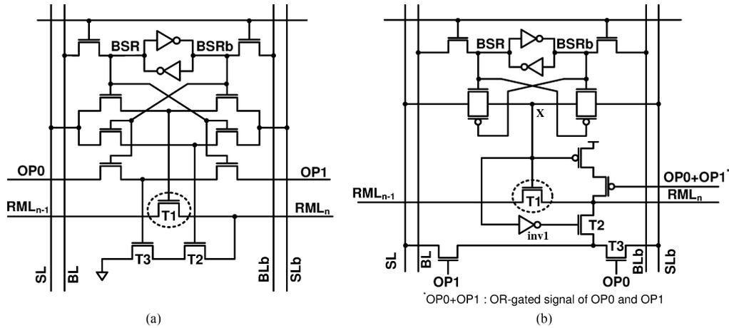
Fig. 6. (a) RMC with a dynamic match-line structure. (b) RMC with a static match-line structure.
