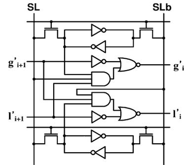
Fig. 5. Range-check cell of an Extended TCAM [9].
