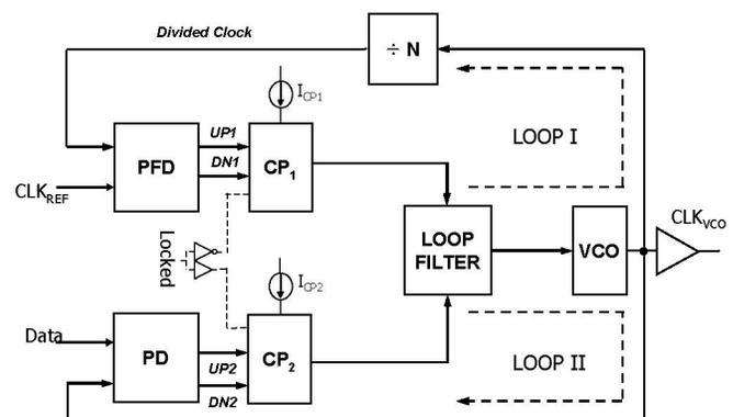
Fig. 1 Clock and data recovery circuit architecture
