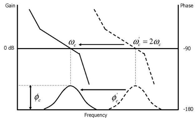
Fig. 3 Bode plot of the open loop response [8], [9]
