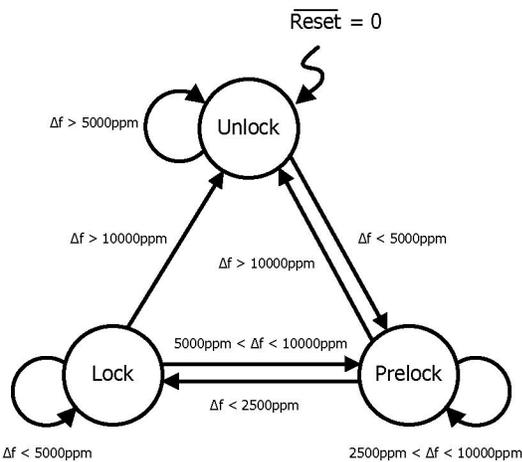
Fig. 2 The state diagram of lock detector
