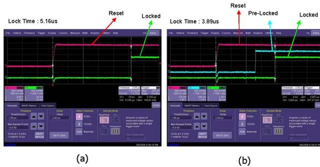
Fig. 7 Comparison of the locking times: (a) CDR without a *PRELOCK* signal (b) CDR with an autonomously reconfigurable structure
