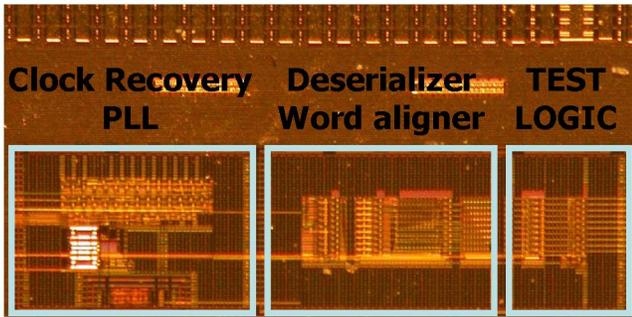
Fig. 6 Microphotograph of the 1.25Gb/s serial link including autonomously reconfigurable architecture
