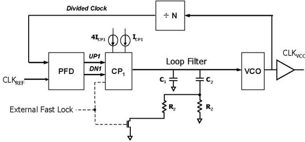
Fig. 4 An existing fast-locking PLL architecture [8]
