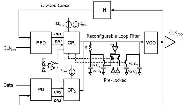
Fig. 5 Autonomously reconfigurable architecture
